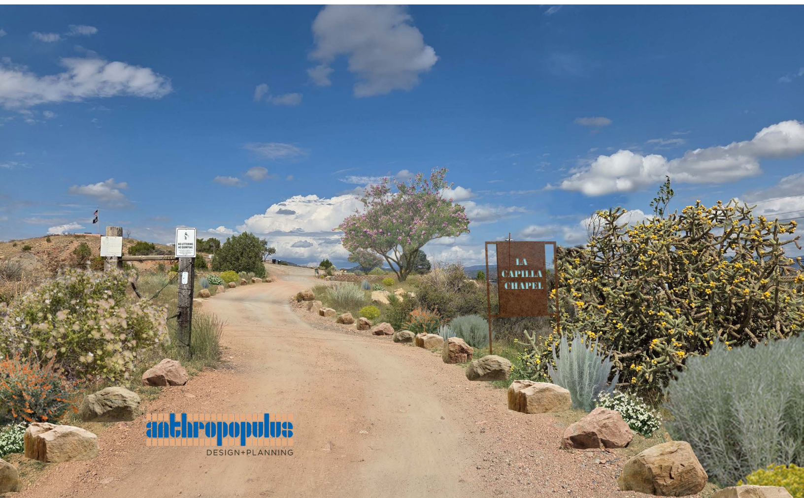
Rendering re-imagining the entrance, parking area and trailhead of La Capilla with additional trees and native vegetation. Adding GSI features to the road, and directing that runoff to planted areas will help prevent further erosion and irrigate added trees. Renderings by Anthropopulus Design + Planning.
